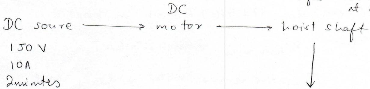
$$\text{Torque} = 230 \text{ Nm at } 60 \text{ rpm}$$
