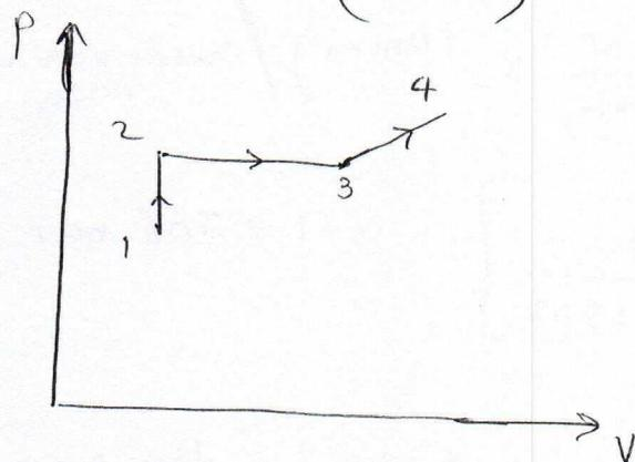
The heating is finally stopped when the spring is compressed by 1 cm (⊕ on the P-V diagram).
