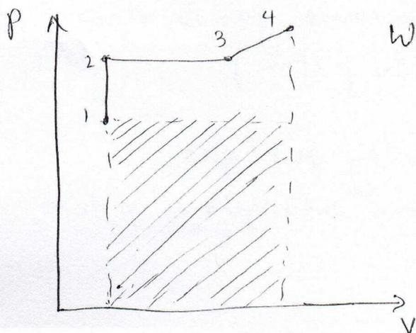
$$\begin{aligned} W_{\text{atm}} &= - (V_4 - V_1) \times P_1 \\ &= - (6.36 - 4.417) \times 10^{-3} \times 10^5 \\ &= -194.3 \text{ J} \end{aligned}$$
